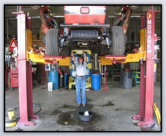
The Mohawk Turf Package has allowed for ground care maintenance vehicles to be lifted easily to the height of six (6) feet. The mechanic now has unrestricted under-vehicle access while standing to perform repairs and maintenance.
