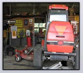
Tractor mowers such as the one in this photo were lifted by a floor jack to be serviced. The mechanic was required to lie on the ground under the mower in order to perform repairs and maintenance.
